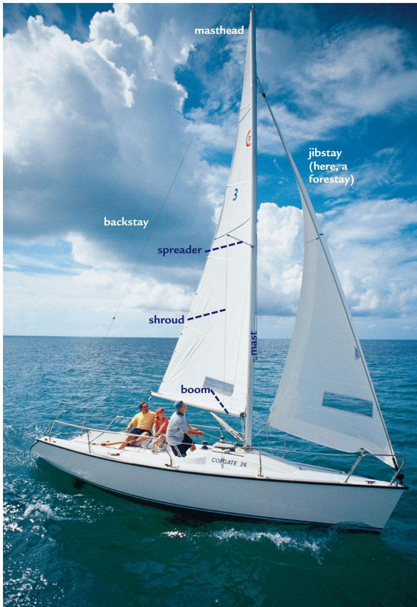
Figure 1-3. Terms that describe standing rigging.
