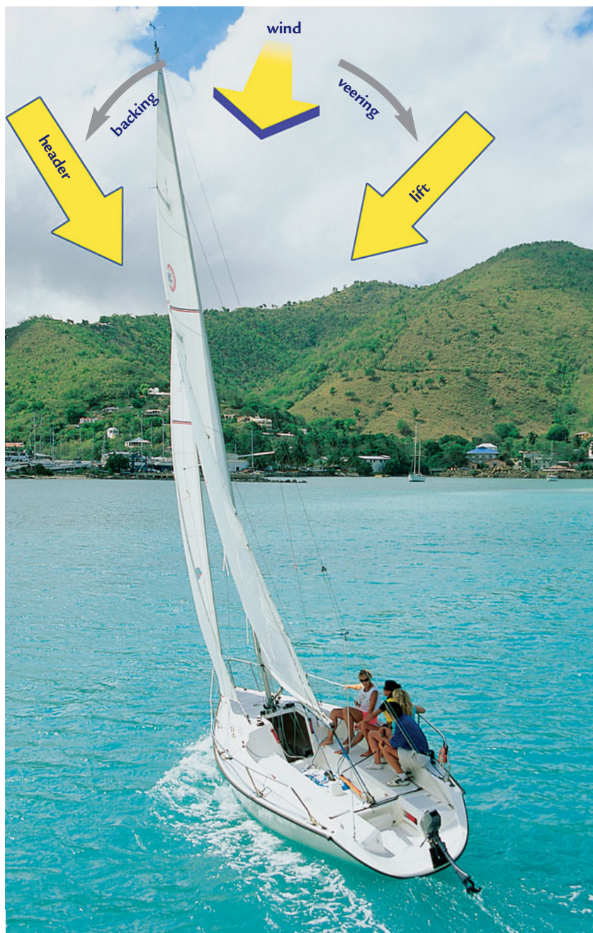
Figure 4-17. A backing wind heads this boat while a veering wind is a lift.
