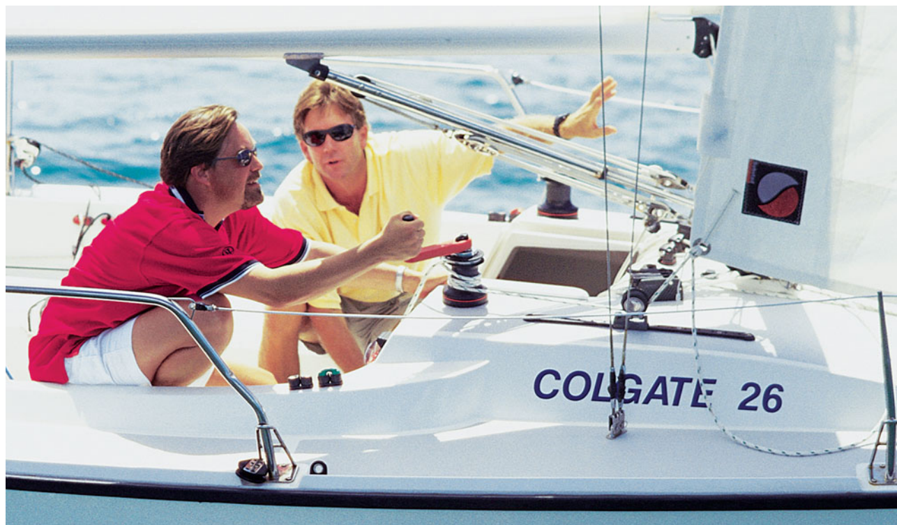
Figure 1-4. Adjusting a jibsheet (running rigging) changes sail shape.
