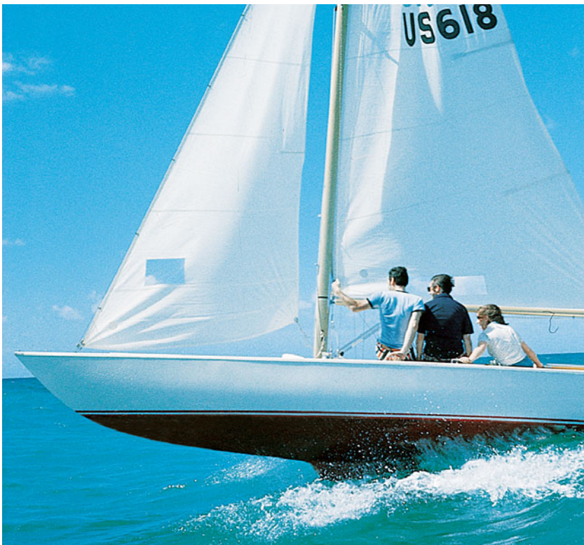
Figure 5-10. When sailboats surf, hull speed is exceeded.
