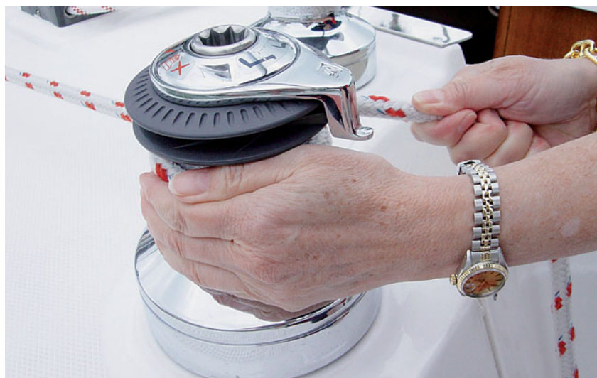
Figure 10-4. Proper way to ease a sheet on a winch.
