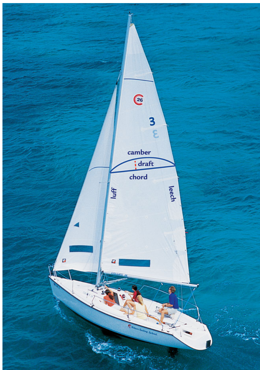
Figure 4-11. Chord, camber, and draft define sail shape.
