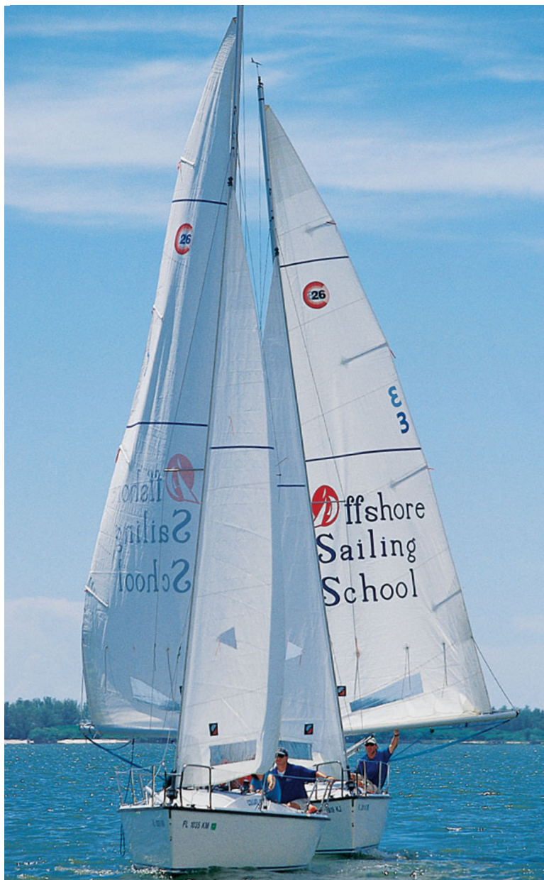
Figure 4-23. Sailing by the lee, with the wind on the same side as the boom, this boat is in danger of jibing.
