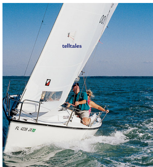
Figure 4-7. When both telltales stream aft, airflow is smooth and even.
