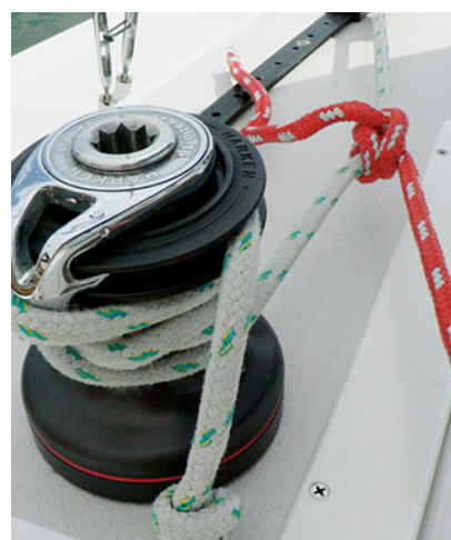
Figure 10-5. Using a spare line, tie a rolling hitch to the line that is jammed on the cleat to relieve the strain, then untangle the wraps on the winch.
