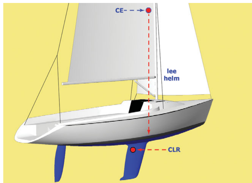
Figure 5-3. Lee helm is caused when CE moves forward of CLR.
