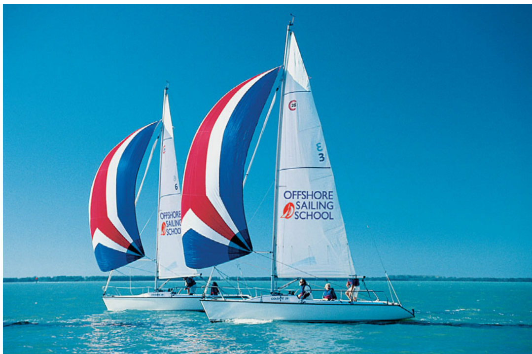
Figure 9-5. Both spinnakers are properly set: tack and clew are level.
