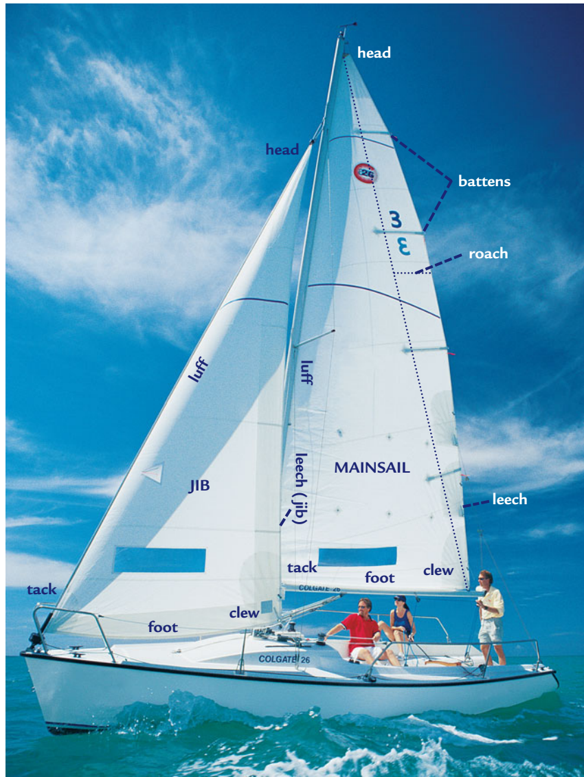
Figure 1-6. Terms that describe the parts of a sail.
